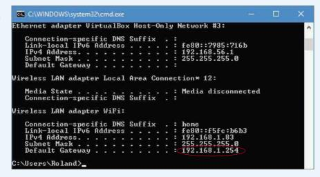
Find the router's IP address with ipconfig at the command prompt
