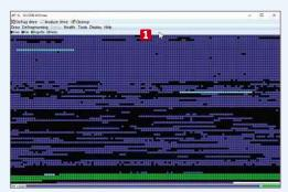
Install Vopt and save the licence key as a TXT file to the folder at C:\Program Files (x86)\Golden Bow\Vopt 9. Run the program and it will analyse your drive and show a colour-coded disk-usage map. 11 Blue squares are file data, black are free, cyan are Windows metafiles, and green are fixed Windows files.
