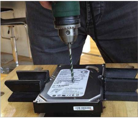
Drilling holes through a drive is one of the most effective ways of destroying it and preventing data recovery
